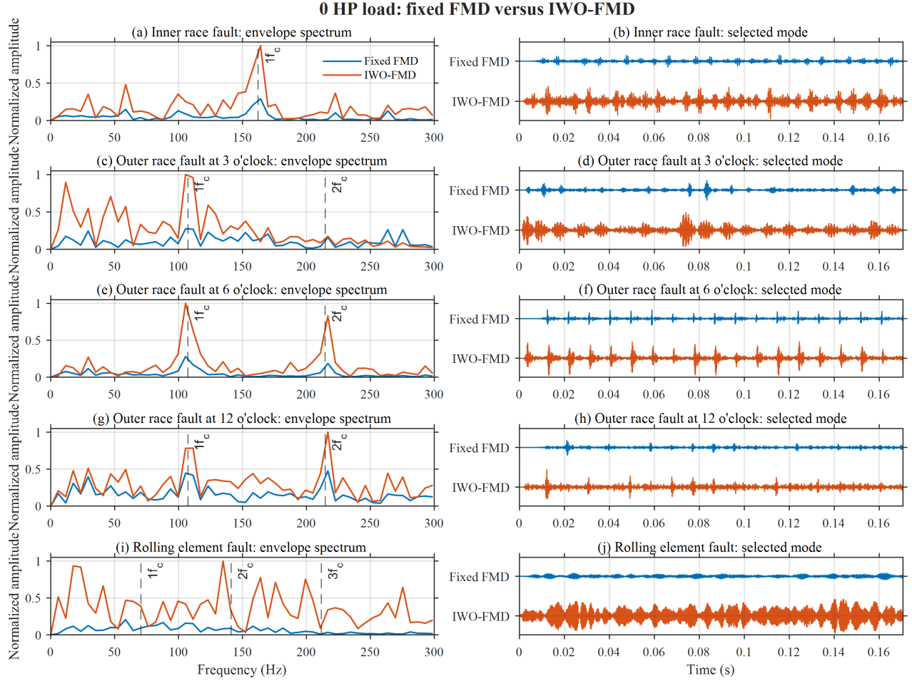
Fig. 4. Comparison of envelope spectra and fault-sensitive modes under 0 HP load
